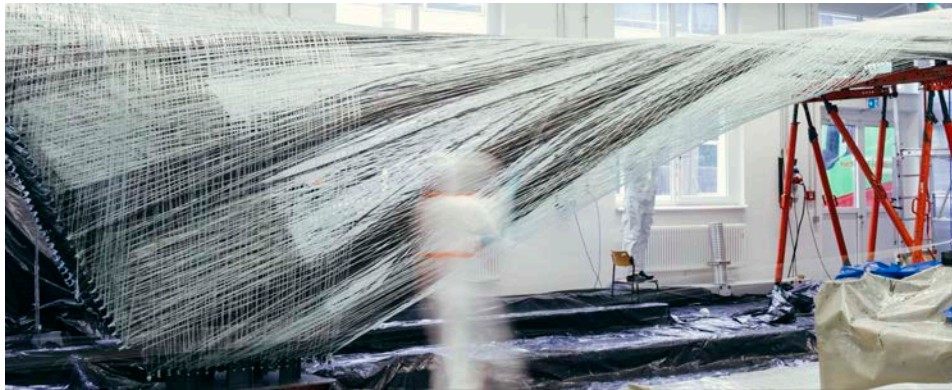
Figure 5: Glass fibre body of the cantilever with initial carbon fiber strands
